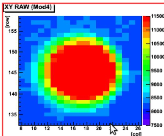
The distance between DEPFET matrix and laser nozzle for such focus is in vicinity of 1.2 cm and it was changed step by step for the 50  $\mu\text{m}$  interval to get the smallest area.
