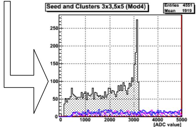
Right seed distribution of the laser appears at 4000 ADC after plugging in the pulse, together with fetched in noise from previous emitting. That is why, it is necessary to calculate the pedestals first and then run data acquisition with calculated pedestals after laser is powered and pulse is applied to it.
