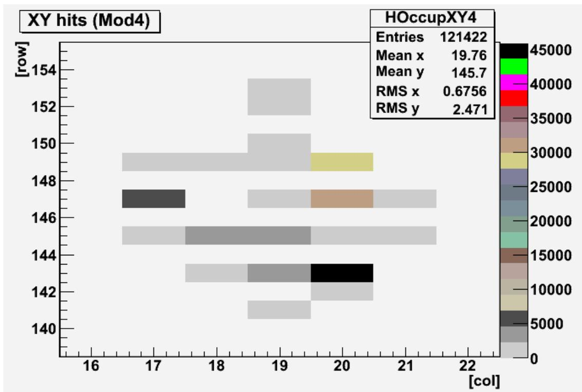
As it can be seen from 'XY hits' plot, laser beam is not perpendicular to the matrix and beam is not concentrated in one or few neighbor pixels!
