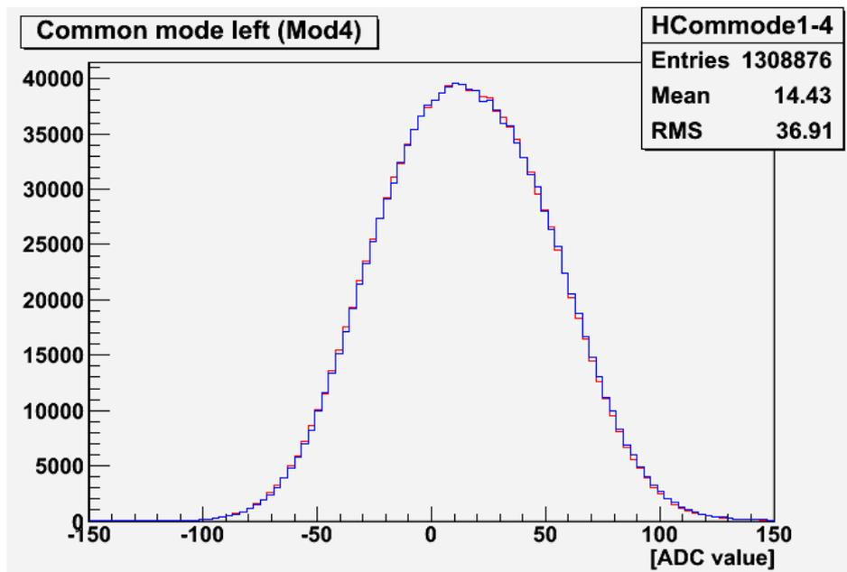
So, DEPFET matrix H 3.0.13 is suitable for data acquisition instead of many bad pixels. It has rather low noise, stable pedestals and content common mode. Pedestals, obtained during this run (run number 9999), are used and will be using for further runs with different radiation sources and laser.
