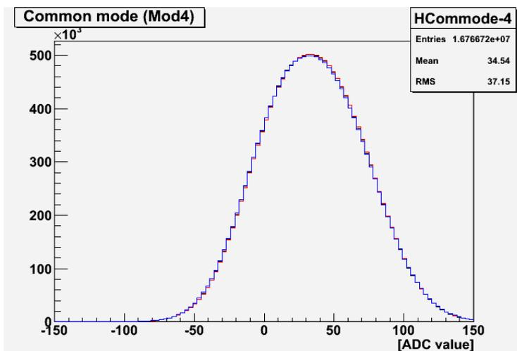
Still spectrum is almost the same and the common mode is shifted to the right (34.5 ADC). Maximum *Clear\_high* voltage is 10.4V, so maximum reasonable *Clear\_low* voltage is 10.2V. Also, it is not recommended to apply greater than 7V *CCG* voltage as it was mentioned previously.
