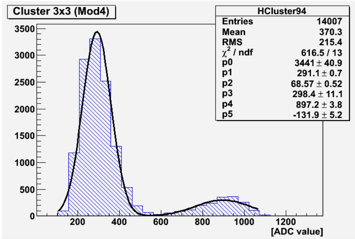
There are only two peaks. One peak couldn't be seen (probably) because of the noise as  $6\sigma$  cut was done and first ~108 ADC units were removed. Therefore, we can see only second and third peaks (???). Still the ratio  $p4/p1$  is 3.08. Besides that, amplitude of the second peak is 11.5 times bigger than third one.
