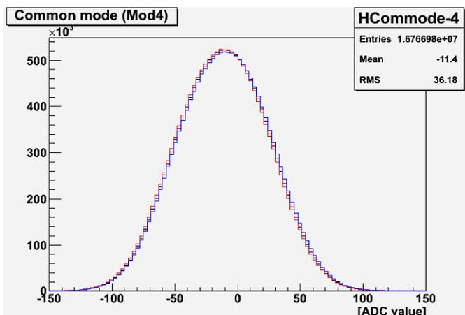
Common mode's mean value is around 0 (shifted to the left by 11.4 ADC) and the spectrum is similar to standard situation.
