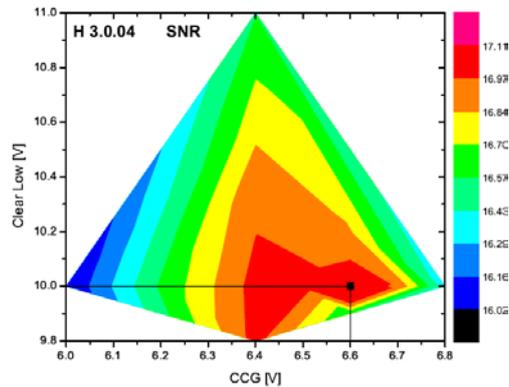
Standard value (for matrix H.3.0.13) for *Clear\_low* voltage is 10V, for Common Clear Gate (*CCG*) – 6.4V. Don't forget, that there is no *Gate\_on* voltage!
