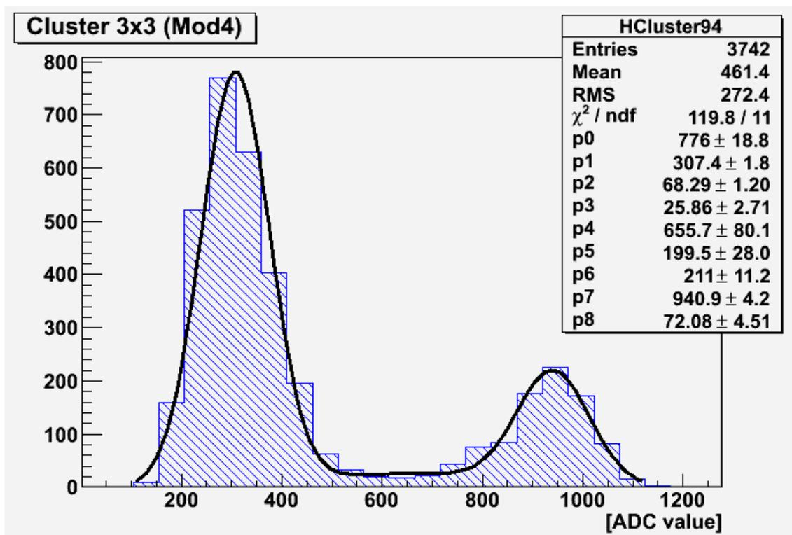
There is no significant reduction of the first peak, as it was expected from the calculations, but the constant of the peak is falling-off for several times. Also, it can be seen not well defined third peak in the middle.
