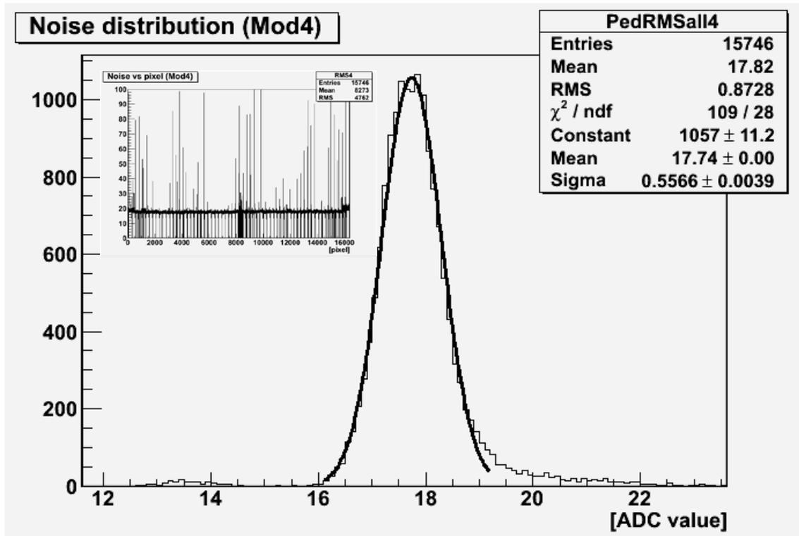
Mean value of the noise distribution is 17.74 ADC. All other same matrixes, those are at Bonn or Munich for the present moment, have mean value around 14-16 ADC units. Should be mentioned, that these matrixes are clean (there are no bad pixels) and only one single bad column of pixels can increase noise up to 17 ADC (matrix H 3.0.10).
