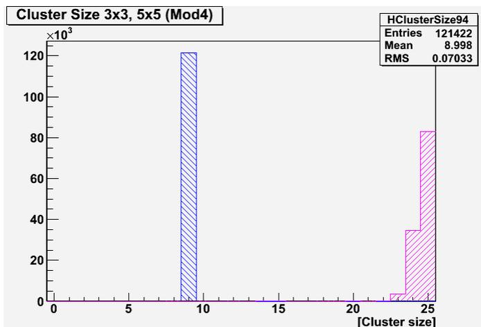
It is necessary to analyze cluster 10x10 for the present case, but cluster 3x3 should be enough after good focusing of the laser.
