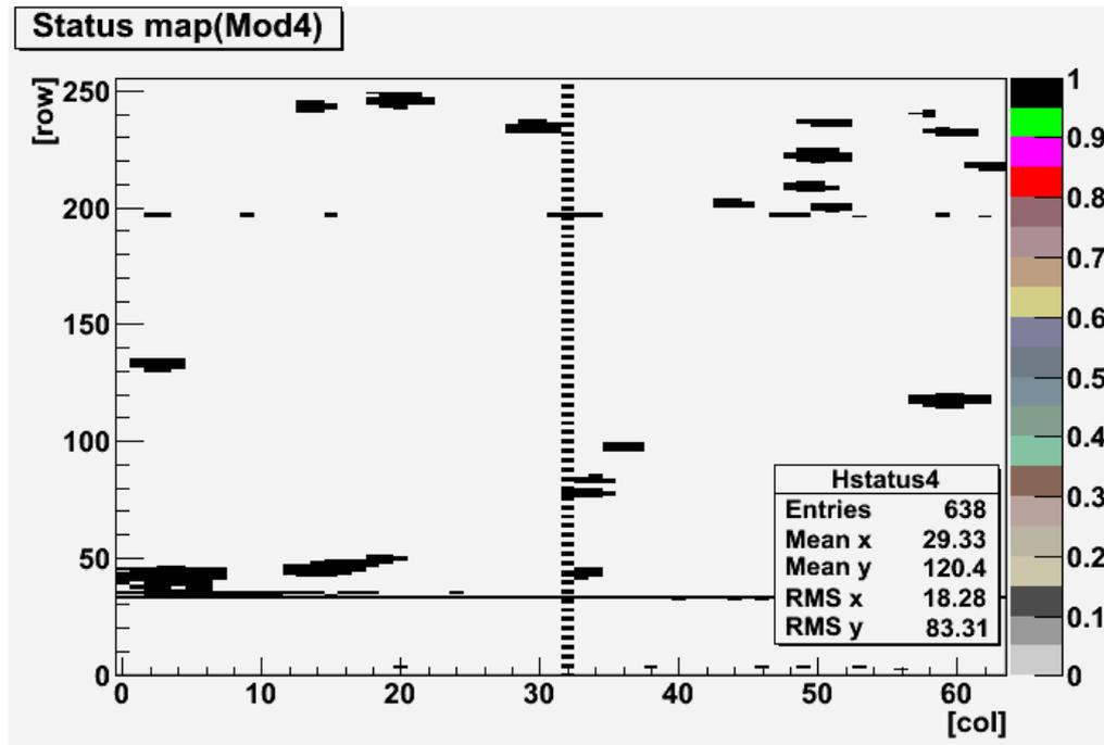
So this DEPFET matrix has around 3.9% of bad pixels, most of them are calculated by the software and also about 20% were selected during the test runs with further masking by hand.
