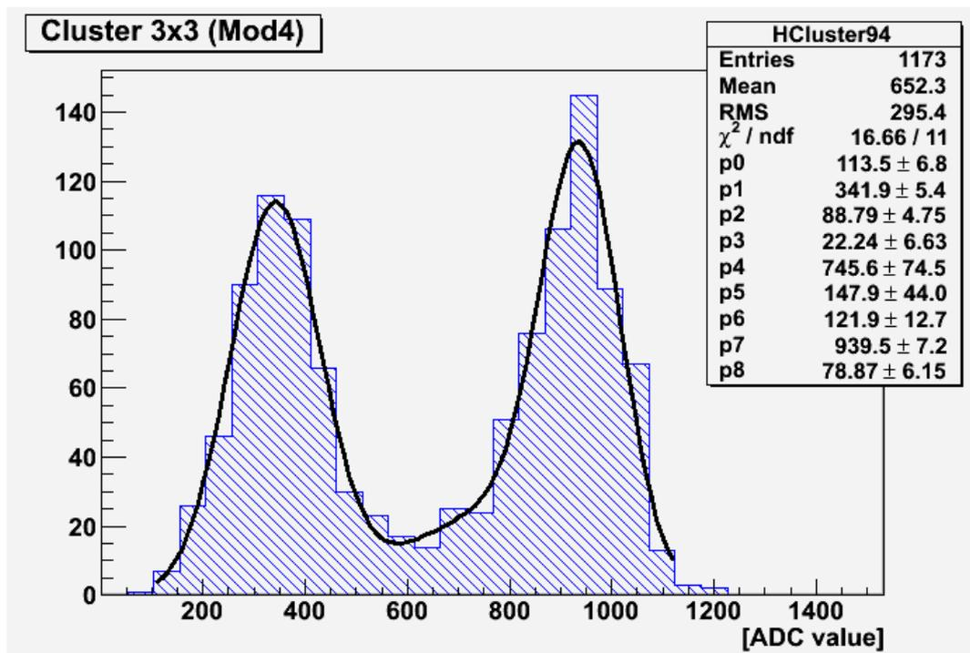
Eventually, the third peak is greater than the first one and it is possible to evaluate the second one: constant of amplitude is around 22 (p2), mean value 745 (p4) with sigma almost 150 (p5). The most important peak of 60 keV is at 939 ADC with the constant 122. Ratio between the first and the last peak is 2.75.
