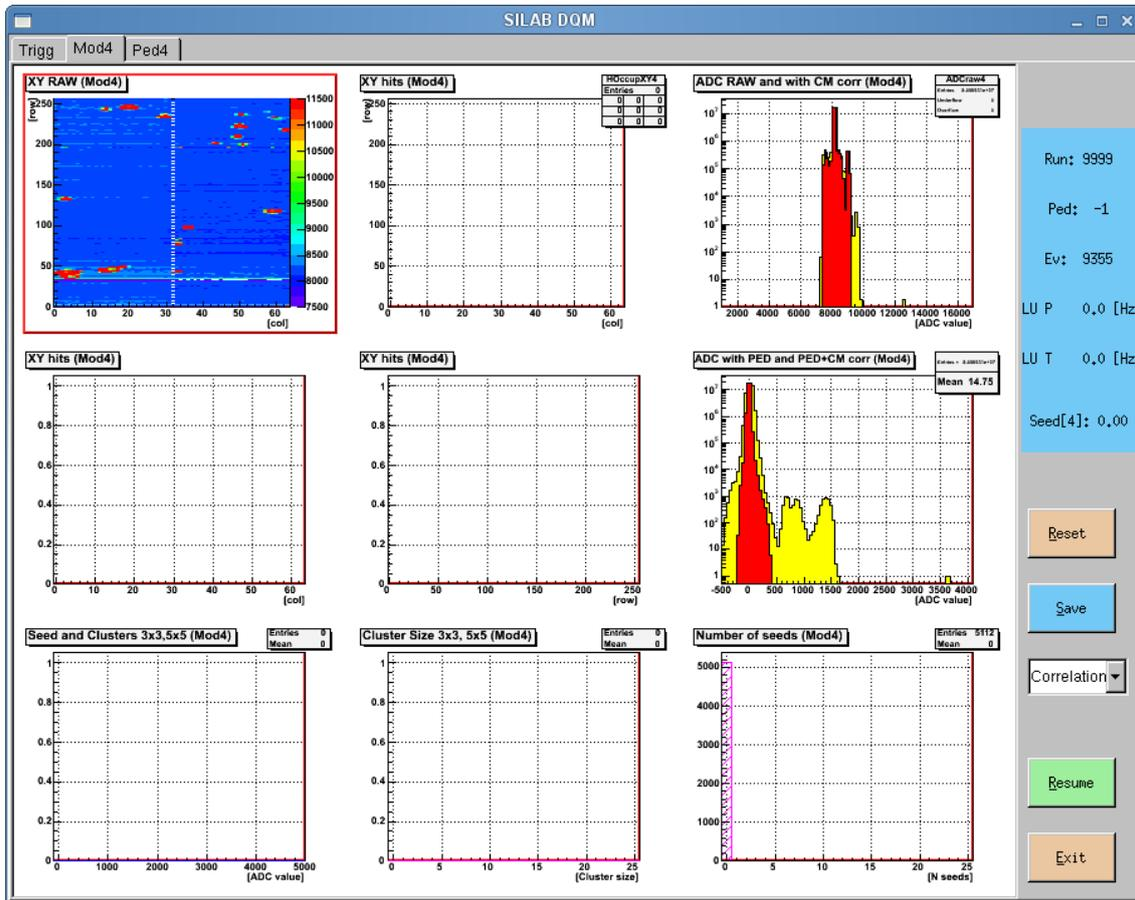
As there are no interactions of particles with the matrix, all 'XY hits' plots, plot of energy of one seed, 'Clusters' and 'Cluster Size' plots are empty. Also it can be seen 0 seeds in the 'Number of seeds' plot with 5112 entries.
